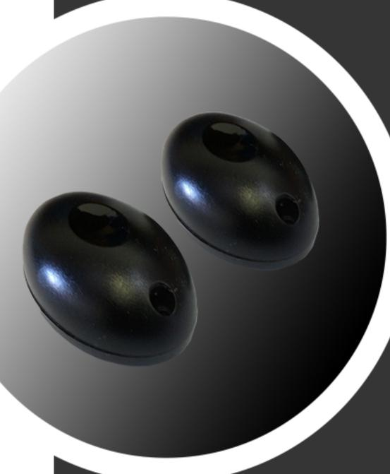
Designed to increase safety on vehicles, children and even pets, the photo beam sensors are placed (one on each side) between the opening. During operation if the beam is interrupted/ broken the automation unit registers and reverses its operation, avoiding any collision resulting in damage.
