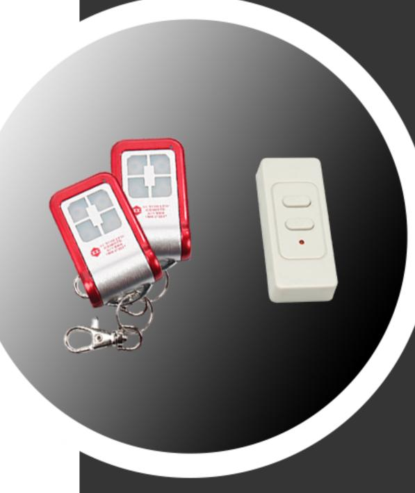
The ARA Transmitters work on the unique frequency channel of 433.22mhz with a rolling code providing over 1.2billion different combinations for your peace of mind. The wireless wall mount (two channel transmitter) and the keychain handheld transmitter (four channel) allow multiple units to be paired to the one control.
