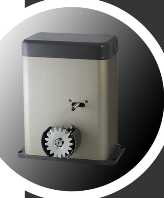
Domestic Sliding Gate Motor is the ideal unit, quiet in operation, quick in movement (approx 13.3m per minute) and heavy duty moving gates that weigh up to approx. 500kg! The PY500AC operates via forcing a drive rack by a drive gear.
