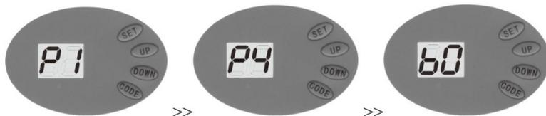
Press and hold **SET**, LCD displays "P1", press **UP** three times, it displays "P4". Press **SET** to show current situation. Press **UP** to increase the Auto-close one minute and press **DOWN** to decrease one minute. Maximum degree is "b9" and minimum is "b0". Press **SET** to confirm. The default setting is "b0". "b0" shows auto-close off.
