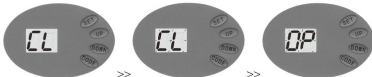
Display will show "**CL**", then press **DOWN**, it displays "**CL**". When the door has reached the closed position, press **SET**.
