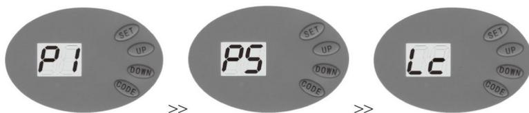
Press and hold **SET**, LCD displays "P1", press **UP four times**, LCD displays "P5", press **SET** to show current situation. Press **UP**, it displays "Lc", lock door function works, press **DOWN**, LCD displays "uL", the lock door function doesn't work. Press **SET** to confirm the function you need.
