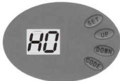
Press **down** once, LCD displays "H0", the photo beam is disabled. Press **SET** to confirm and quit.
