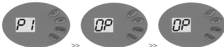
Press and hold **SET** until it displays "**P1**", press **SET**, it displays "**OP**". Then press **UP**, when the door has reached the open position, press **SET**.
