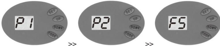
Press and hold **SET**, LCD will display "P1", press **UP** once, it displays "P2", press **SET** once again, it will show the current situation. Press **UP** to increase the force one degree and press **DOWN** to decrease one degree. Maximum degree is "F9" and minimum is "F1"
