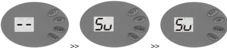
Press **CODE**, it displays “Su”, press a button on the transmitter, then release and press the same button again, “Su” flashes, then it displays “- -” to show setting is complete.
