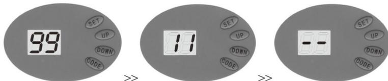
Turn on the power, The LED displays from **99** to **11**. At last, it displays " - - - "
