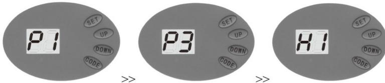
Press and hold **SET**, LCD displays "P1", press UP twice, it displays "P3". Press **SET** to show current situation. Press **UP** once it displays "H1", the photo beam is enabled.
