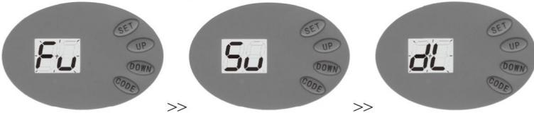
When unit displays “Fu”, press and hold **CODE** more than **8** seconds until it flashes “dL”, all the codes will be cancelled.
